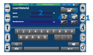
After registering or modifying a load, the load list will be displayed for 4 sec. and then return to the job.
