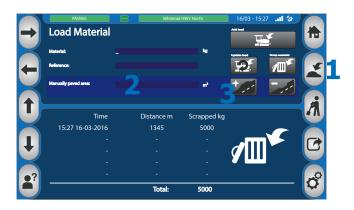
After adding the manually paved area, a list of manually paved areas will be displayed briefly on the bottom screen. The list can also be accessed by using the arrow buttons right and left, when in the "Load" menu.
