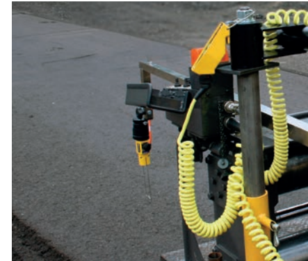
Mini-Line® regulates with mm-precision. Here is seen HS301 and the grade sensor furthest back on the Averaging Beam.
