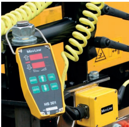
The HS301 handset has a metal hanger, so that the operator can easily hang it on the paver.
