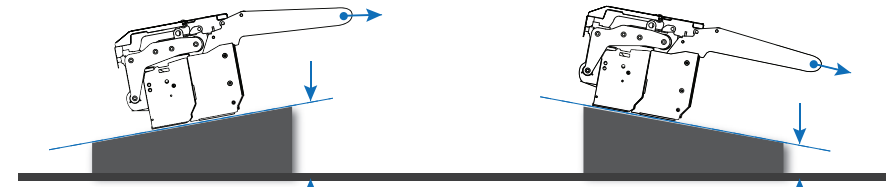
Figure 2 - Increase in angle of attack - increased mat thickness
