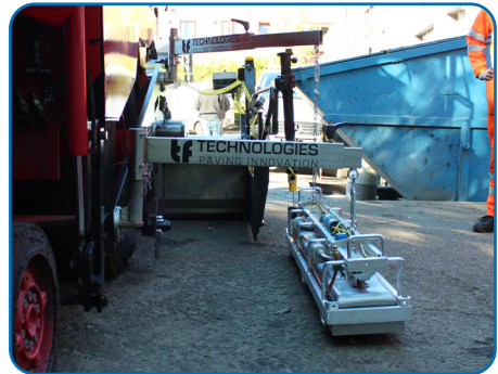
Fig. 4 - Joint Heater Mounted on mounting arms on a machine
