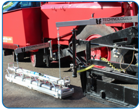
Fig. 3 - Joint Heater Mounted on mounting arms on a machine
