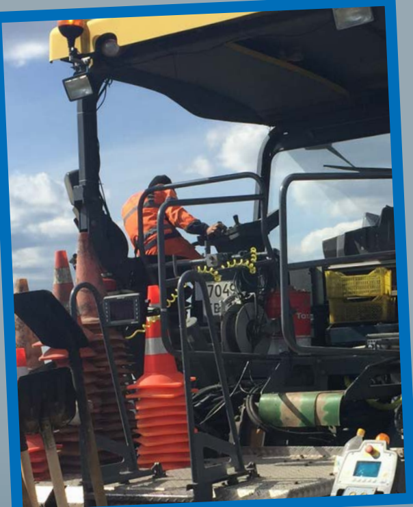
MatManager™ on a Vögele SUPER 1900-2 paver
