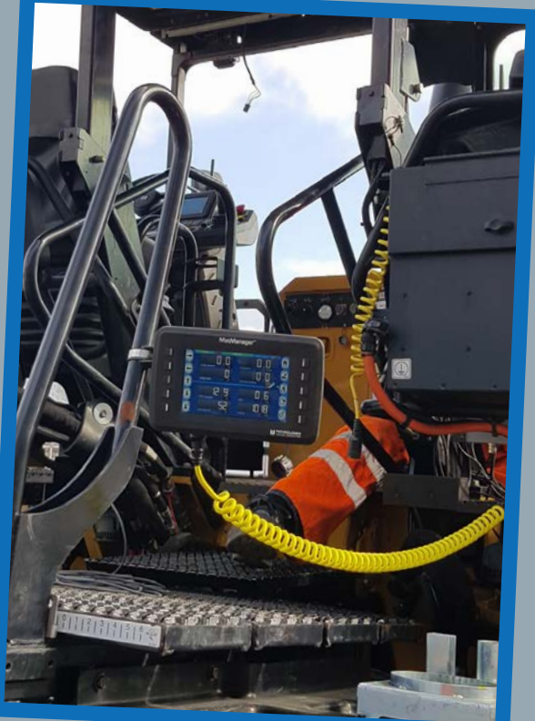
MatManager™ installed on a CAT AP655F
