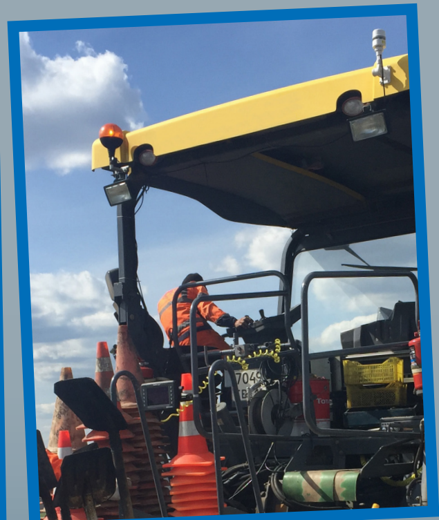
MatManager™ on a Vögele SUPER 1900-2 paver
