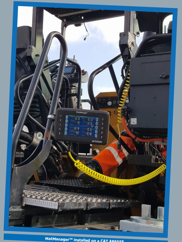
MatManager™ installed on a CAT AP655F
