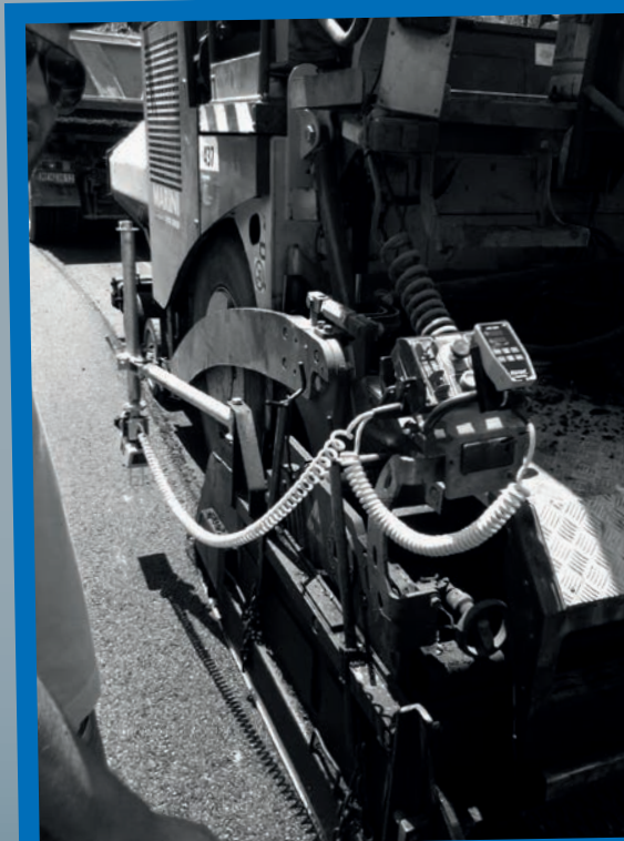
Mini-Line® HS301 Grade Control Kit with G224
