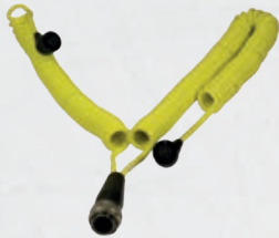
V-Cable V-Cable with one 10-Pin Screw, and two 6-Pin Bayonet. Used for connecting the machine to HS301 Handset and Grade Sensor or Slope Sensor.
