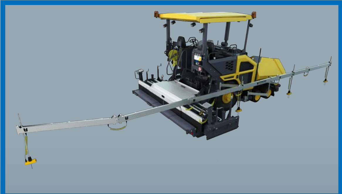
Mini-Line® SUPER Averaging Beam with Hinge, 13m / 40 ft on paver
