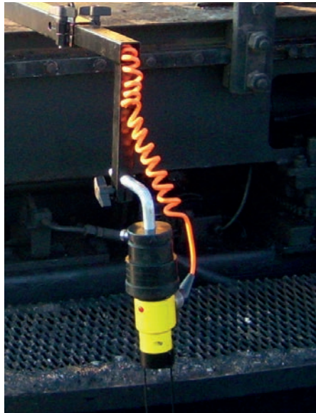
The sensors are connected by the internal cabling of the Averaging Beam.
