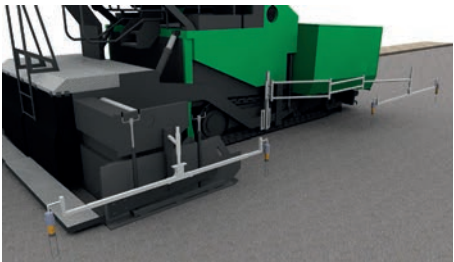
Asphalt paver with Averaging Beam and four grade sensors.
