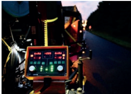
The PL2005 automatically adjusts the brightness of the LED display for bright or dark surroundings.
